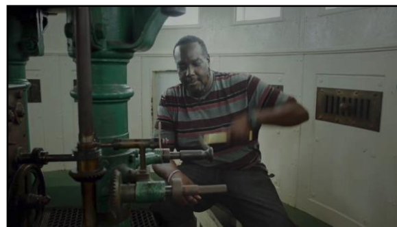
Elbow Reef Lighthouse Keeper Jeffery Forbes Jr. cranking the lens rotation mechanism by hand.
